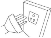
Avoid unstable power sources. Do not operate near large users of electricity such as welding equipment or large motors. Do not let the balance battery go flat – if you are not using it for a long time you should charge the battery up periodically to make sure the battery dose not lose its charge.
