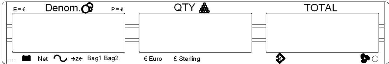
The **Denomination** window shows the current denomination that has been selected, an arrow will indicate when the scale is at zero (**ZERO**) and when the weight is stable (**STAB**) or if the scale has been tared (**Net**) and is displaying a net weight. An arrow will show if a bag weight has been selected.
