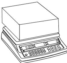
Keep the scales clean, and do not stack material on the scale / balance when it is not in use.
