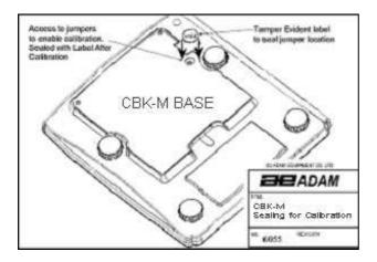
The calibration of the CBK-M scale is accomplished by removing the label at the base of the scale which covers a hole through which the PCB can be accessed. If your scale is not provided with this hole, you need to break the security seals and remove the top cover to gain access to the circuit boards inside. See the figure on the security seal below.
