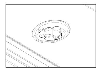
To seal the scale a lead-wire seal can be used as shown below. The base has a metal pin that protrudes through the cover. The security seal may be threaded through this metal pin, making it impossible to remove the cover without damaging either the security seal or the enclosure.
