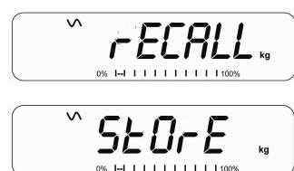
If you want to store the limits, when “StOrE” is displayed press the [Tare] key. The display shows “St ”. Enter a number corresponding to the desired memory location (0 to 9). “St X” will be displayed for 2 seconds indicating the location X where the current limits, weighing units and settings for the beeper and bar graph are stored. The indicator will continue to work with the current settings as active.
