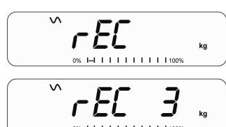
displayed. The display shows “**REC**”. Enter the number corresponding to the desired memory location (0 to 9) to be recalled. “**REC X**” will be displayed for 2 seconds indicating the values stored in the location “X” is being recalled. The indicator will change to the recalled limits, weighing units and settings for the beeper and bar graph.
