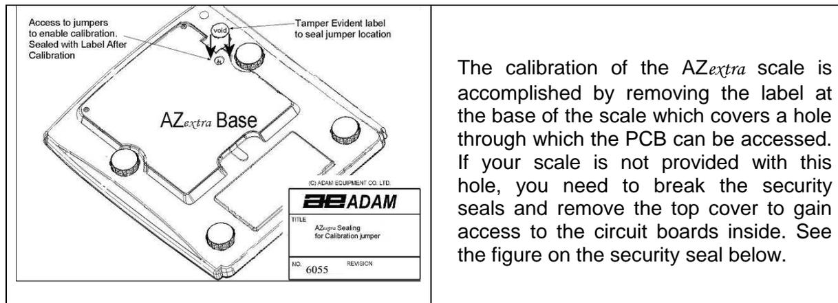
The calibration of the *AZextra* scale is accomplished by removing the label at the base of the scale which covers a hole through which the PCB can be accessed. If your scale is not provided with this hole, you need to break the security seals and remove the top cover to gain access to the circuit boards inside. See the figure on the security seal below.
