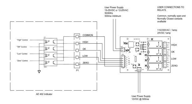
Connections to the AE042 are made at terminal strip P1:
